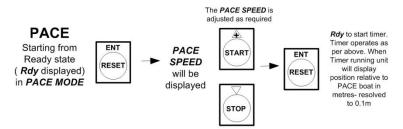
Rate and Speed will be displayed on top line. The default display on bottom line is distance: +/-metres from PACE boat on left and TIME on right. See display options in General Operation section, if you wish to display o
