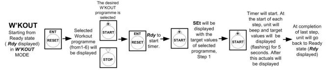
Note: If *Ent* button pressed during workout, programme will hold, and HOLD will be displayed. Pressing *Ent* again will release HOLD. This feature is handy if you have to stop during your workout, eg to make a turn.
